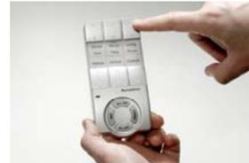
3. Select your INSTEON Device from the list below and follow the linking method for that Device. You have about 4 minutes to perform this step before RemoteLinc's Linking Mode times out automatically.
