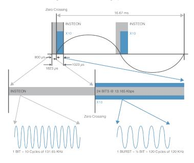
The top of the figure shows a single powerline cycle, which possesses two zero crossings. An INSTEON packet is shown at each zero crossing. INSTEON packets begin 800 microseconds before a zero crossing and last until 1023 microseconds after the zero crossing.
