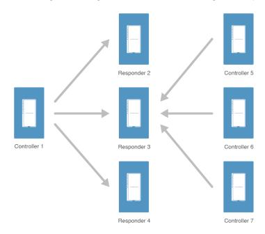
Any non-battery-powered INSTEON device can repeat<sup>1</sup> messages, as with device **B** below, which is shown relaying a message from device **A** acting as a controller to device **C** acting as a responder.
