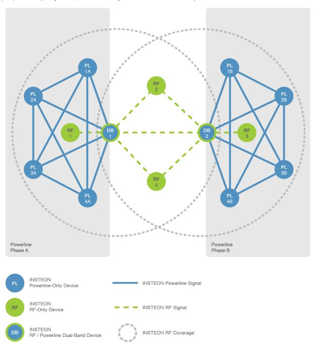
Every INSTEON device is capable of repeating INSTEON messages. They will do this automatically as soon as they are powered up—they do not need to be specially installed using some network setup procedure. Adding more devices increases the number of available pathways for messages to travel. This path diversity results in a higher probability that a message will arrive at its intended destination, so the more devices in an INSTEON network, the better.
