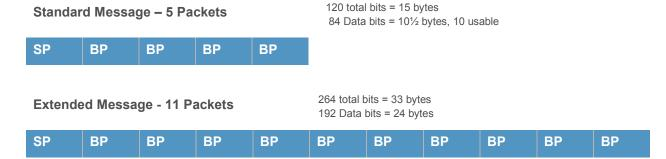
Each packet contains 24 bits of information, but the information is interpreted in two different ways, as shown below.
