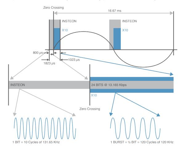
The top of the figure shows a single powerline cycle, which possesses two zero crossings. An INSTEON packet is shown at each zero crossing. INSTEON packets begin 800 microseconds before a zero crossing and last until 1023 microseconds after the zero crossing.
