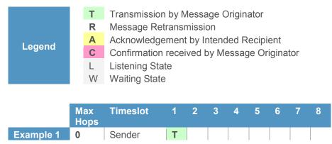
**Example 1**, the simplest, shows a Broadcast message with a Max Hops of zero (no retransmissions). The **T** indicates that the Sender has originated and transmitted a single message. There is no acknowledgement that intended recipients have heard the message. The message required one timeslot of six or thirteen powerline zero crossings to complete.
