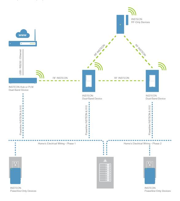
Electrical power is most commonly distributed to homes in North America as split-phase 220-volt alternating current (220 VAC). At the main electrical junction box to the home, the single three-wire 220 VAC powerline is split into a pair of two-wire 110 VAC powerlines, known as Phase 1 and Phase 2. Phase 1 wiring usually powers half the circuits in the home, and Phase 2 powers the other half.
